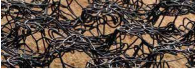
Cedar Breather® is a hard nylon mesh ¼" thick that allows continuous airflow under the shakes.
